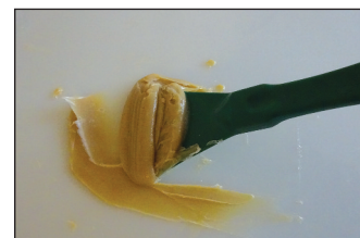
Thoroughly mix DESOWOOD RAP - 4 Hours
